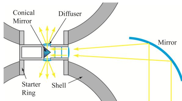
**Figure 5. A passive internal illumination system.**
