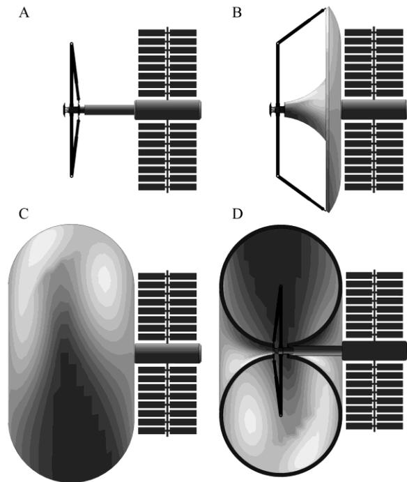
**Figure 4. Three stages of constructing a torus. Starting configuration A, after one third of the outer shell is built B, and after the shell is complete C. D shows a section view of the finished shell.**
