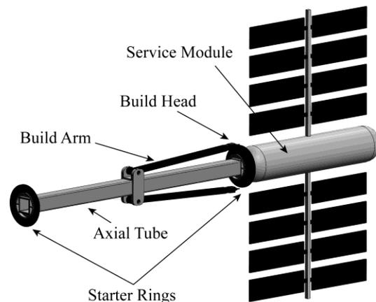
**Figure 1. A simplified representation of a sphere building machine.**
