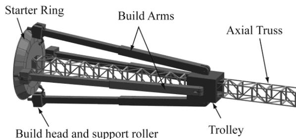
**Figure 7. Detail of the build mechanism.**
