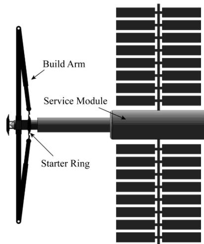
**Figure 3. A torus construction machine in its starting configuration.**
