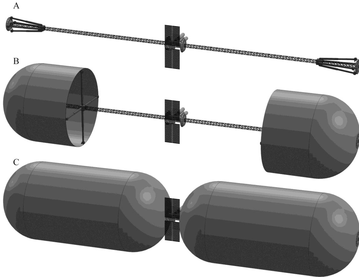
**Figure 6. A kilometer scale habitat at three stages of construction.**
